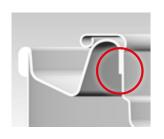
Rolled ring (rolled to the outside)
